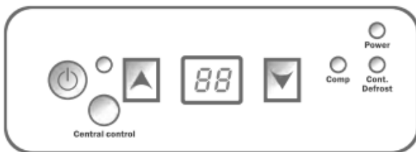
Figure 5. Dehumidifier Control Panel
